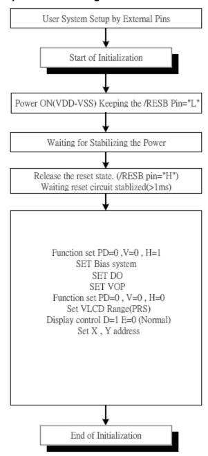
Initializing with the Built-in Power Supply Circuits
