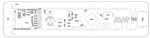
Figure 8-3. AVR128DB48 Curiosity Nano Assembly Drawing Bottom
