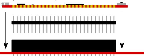
Figure 5-3. Connecting to Curiosity Nano Base for Click boards
