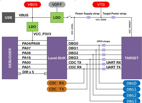
Figure 8-6. On-Board Debugger Connection Cut Straps
