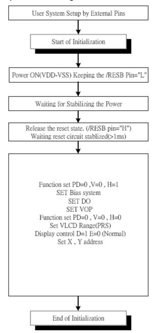
Initializing with the Built-in Power Supply Circuits
