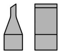
XT Soldering head 10 x 4 mm, spare
