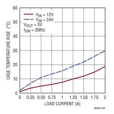
Figure 4. Case Temperature Rise vs Load Current
