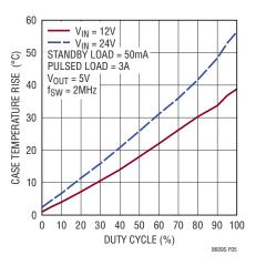
Figure 5. Case Temperature Rise vs 3A Pulsed Load
