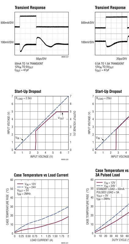
**Transient Response** 8609S G28 20µs/DIV 0.5A TO 1.5A TRANSIENT  $12V_{IN}$  TO  $5V_{OUT}$   $C_{OUT} = 47 \mu F$
