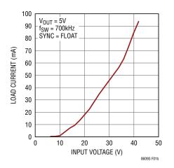
Figure 1b. Full Switching Frequency Minimum Load vs V<sub>IN</sub> in Pulse Skipping Mode
