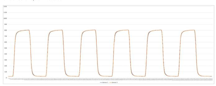
The test results show that repeatability error range <10ppb (2000ppb full scale  $\pm$  1% is the normal range);
