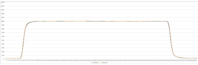
Test results: 2 hours ventilation, range drift <20ppb;
