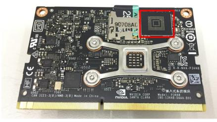
Jetson Nano module with SD Card slot. You can see the SD Card slot easily, as well as the lack of eMMC storage in the highlighted area.
