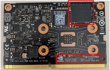
Jetson Nano module with eMMC storage. Note the eMMC module in the highlighted square as well as the missing SD Card slot next to it.
