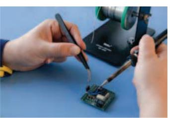
Tweezers are important tools for any electronics technician to enable the necessary work to be carried out safely in the often small, confined structures of PCBs.
