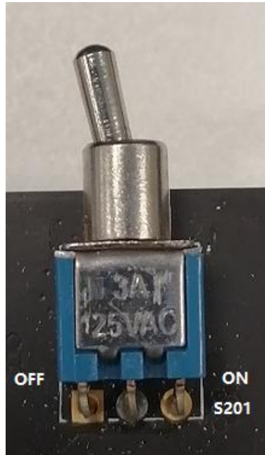
Figure 4: S201 Power Switch
