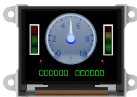
µOLED-160-G2: 1.7", 160x128, 65K colour OLED module
