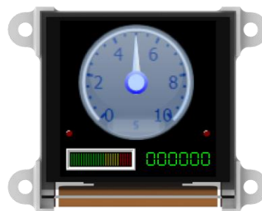
µOLED-128-G2: 1.5", 128x128, 65K colour OLED module
