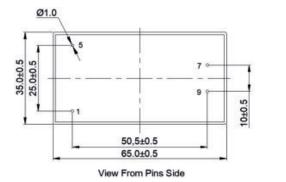
**DIMENSIONS and PINOUT**
