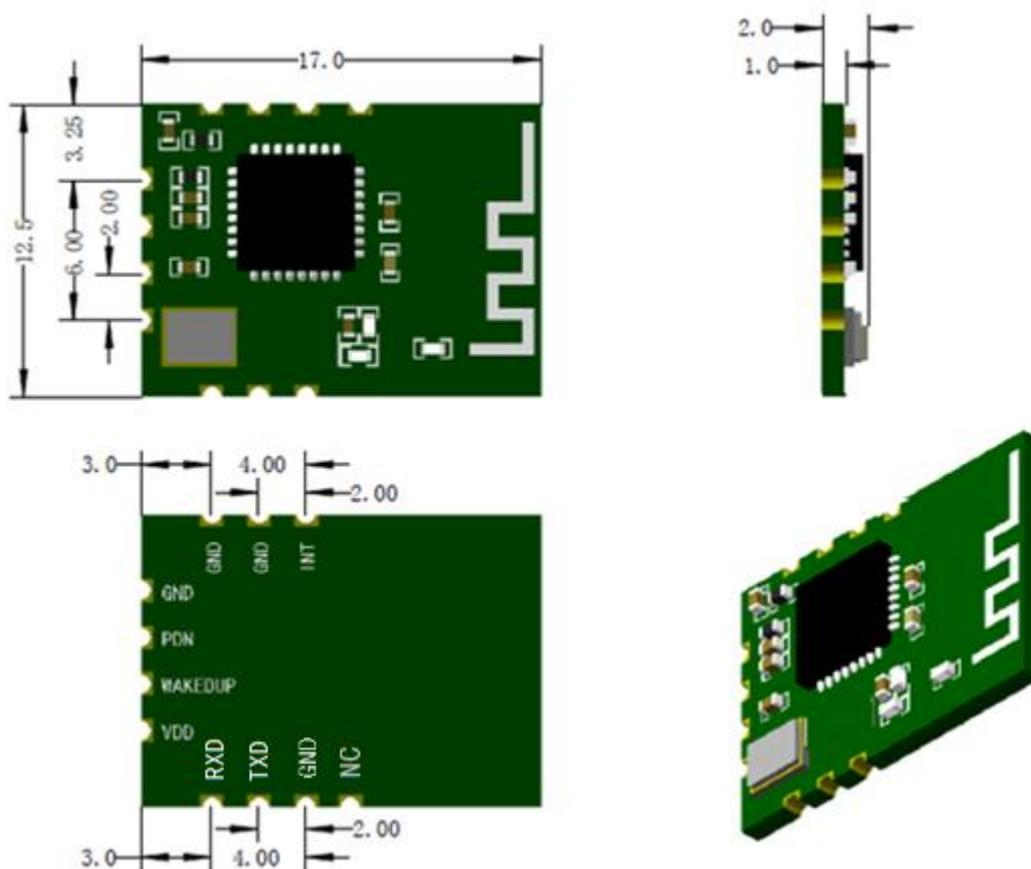
Fig4. Module Size Diagram
