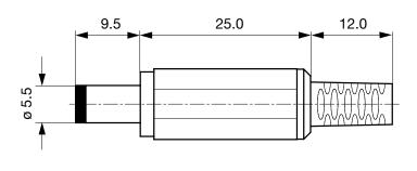
Cable diameter max. 4.0 mm
