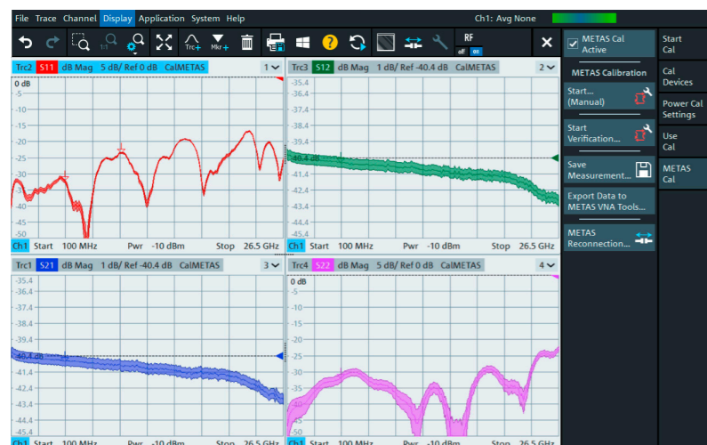
Real-time S-parameter measurements with uncertainty bands.
