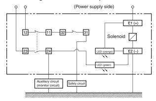
Orange: Lights when the solenoid turns ON. Green: Lights when door closes.
