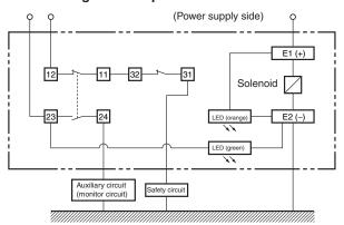
Orange: Lights when the solenoid turns ON. Green: Lights when power turns ON.
