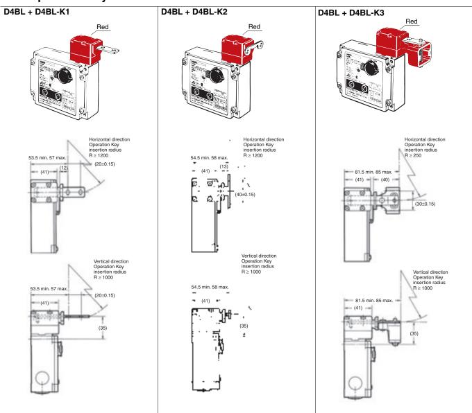
Note: 1. Unless otherwise specified, a tolerance of  $\pm 0.4$  mm applies to all dimensions. 2. In the above diagrams, the Operation Key is inserted from the front.
