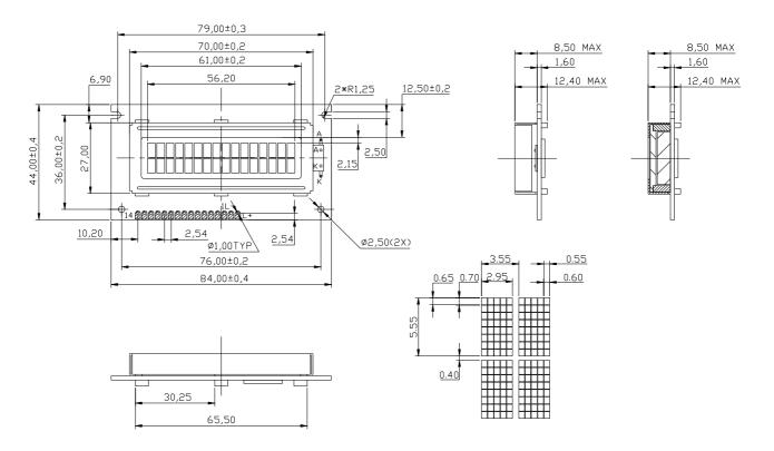
Figure 2.0 External Dimensions For DEM 16217 SYH-LY
