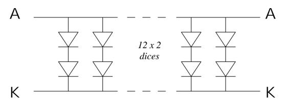
Figure 5.0 Backlight for DEM 16217 SYH-LY
