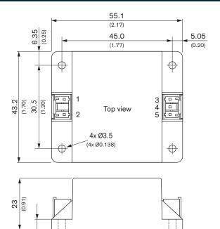
Dimensions in mm (inch) Tolerances:  $x.x \pm 0.5 (\pm 0.02)$
