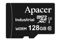
Apacer MSD-WORM Card fully complies with microSD card version 6.1. The command list is compatible with [Part 1 Physical Layer Specification Ver6.1 Final] definitions, while the Card Capacity of Non-secure Area, Secure Area supports [Part 3 Security Specification Ver3.0 Final] Specifications. With built-in ECC, wear-leveling and bad block management, this industrial miscroSD card serves as an ideal portable storage solution.
