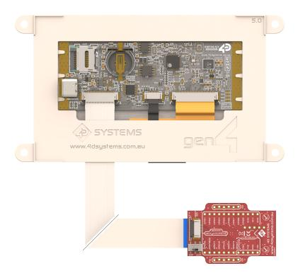
The 4D-UPA is connected to the ESP32 module using the supplied 30-way FFC Cable. The connectors on both the ESP32 module, and the 4D-UPA, are Top-Contact, meaning the FFC cable pins should be facing upwards, and the blue stiffener, should be facing down towards the PCB.
