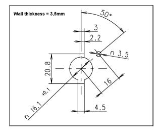
Optional, the sensor can be mounted with a standard Delphi-clip.
