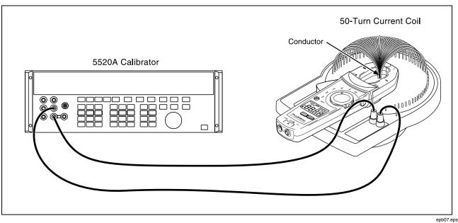
Figure 4. Amps Verification Setup
