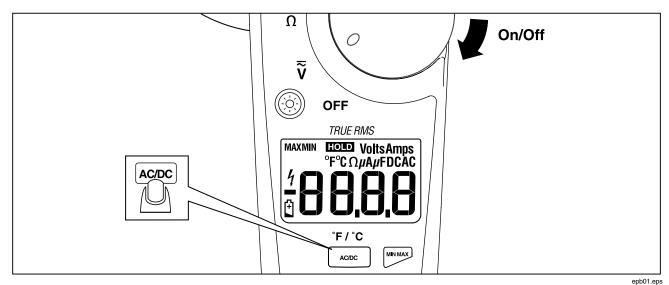
Figure 2. Testing the Display
