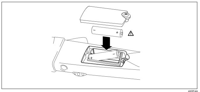
Figure 1. Replacing the Batteries
