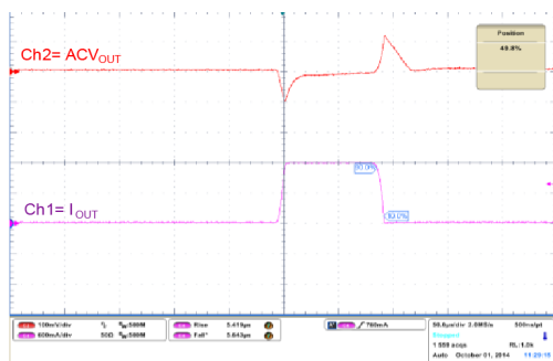
Figure 38. Load transient ( V_{OUT} = 5\text{ V} )
