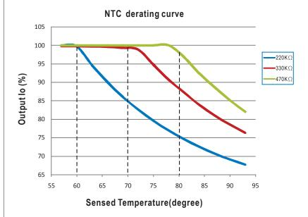
LCM-40EO have the built-in temperature compensation function (T ↑, lo ↓). By connecting a temperature sensor (NTC resistor) between the NTC +/terminal of LCM-40EO and the detecting point on the lighting system or the surrounding environment, output current of LCM-40EO could be correspondingly changed to ensure the long life of LED.
