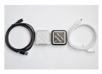
SPS30 USB is an ultra compact (60x60x20mm) Particulate Matter Sensor, which can be directly connected via USB port to PC or embedded system. The SPS30 particulate matter (PM) sensor from SENSIRION used represents a new technological breakthrough in optical PM sensors. Its measurement principle is based on laser scattering
