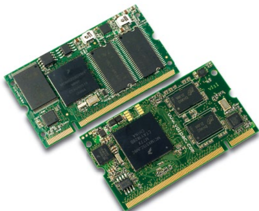
i.MX25 + i.MX51 SODIMM Module (both designed for i.MX25 Base Board)
