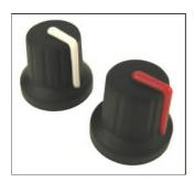
2 colour moulded. 6 standard colours. Soft touch finish. Base Diameter: 16.0 Overall height: 15.0 Shaft depth: 12
