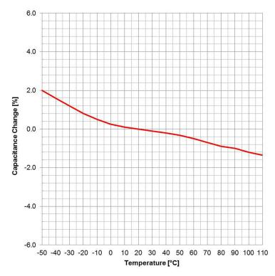
Test Equipment: E4991A or equivalent
