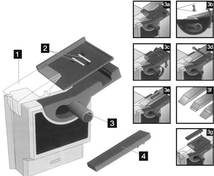
• Position the tool (e.g. a ripping chisel) so that the magnet (2) retains the tool (3a). For small tools, a small plastic insert (4) can be attached on the side so that the magnet is able to retain the tool (3g).
