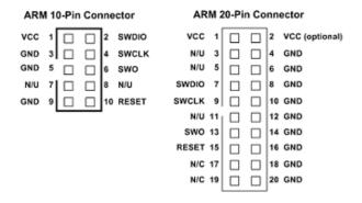
The 3V Pin of ST1 goes to VCC on the Debugger.
