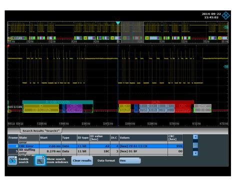
Identifying errors within a serial protocol with the R&S®RTE search function. All events are summarized in a table for easy navigation between different events. Selected events can be zoomed for detailed analysis.
