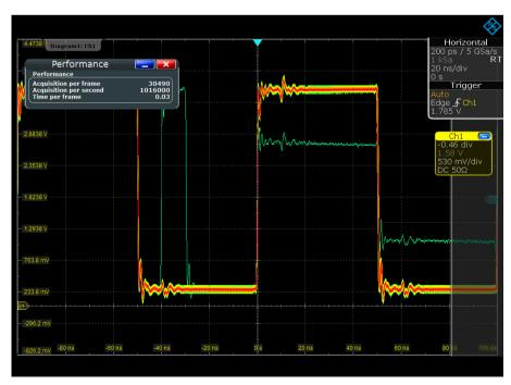
Due to the high acquisition rate of one million waveforms per second, R&S°RTE oscilloscopes find rare signal faults very quickly.
