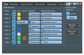
In the R&S®RTE oscilloscopes, up to eight automatic measurements can be configured and activated simultaneously.
