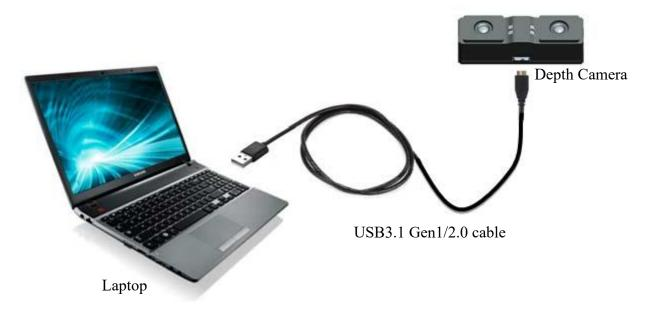
FIG 3-1. DEPTH CAMERA TO PC CONNECTION
