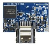
SV250-7LP2 features Apacer Multi-PowerPath technology that provides three methods to supply power to the host either via a conventional cable or cableless design via pin7 or state-of-art 7+2 pin connector, which in turn offers developers maximum flexibility when it comes to board design.
