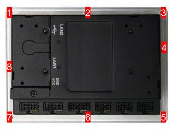
Please follow the steps below to properly install the waterproof rubber O-ring. Prepare your device and O-ring (Step 1-2). First, align the O-ring with the groove and press the O-ring into the corners of the O-ring groove (Step 3-4). Then, press it into the center (Step 5). Finally, stretch it uniformly around the O-ring groove (Step 6). Do not pull from one side, and make sure that you stretch it as little as possible.
