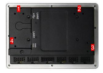
Please follow the steps below to secure the clips. Prepare mounting hook, post and screw (M3) (Step 1). Locate all removable tabs on the rear side of your device and use pincers or pliers to remove the tabs (Step 2-3). Press the mounting clip into the holes at an angle and slowly straighten it (Step 4-5). Then tighten the screw to the surface (Step 6). Repeat the steps for all clips required to secure your device.
