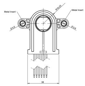
Sensor shown above is the 17mm version with the rotor at zero position. Sensor is delivered at random position. Wires: 0.35mm² TXL SAE J1128
