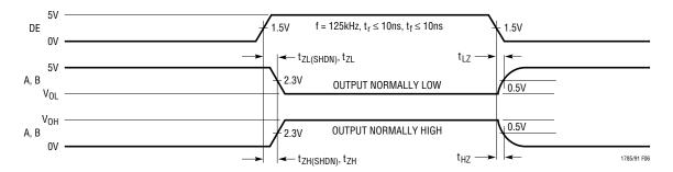
Figure 6. Driver Enable and Disable Times
