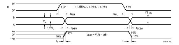
Figure 5. Driver Propagation Delays
