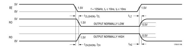
Figure 8. Receiver Enable and Disable Times
