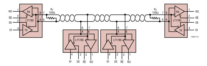
Figure 10. Half-Duplex RS485 Network Operation
