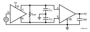
Figure 3. Driver/Receiver Timing Test Circuit
