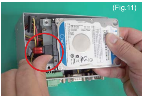
8. Connect the SATA DATA Cable to HDD. (Fig.11)
