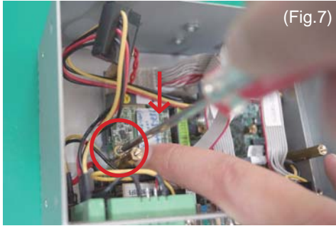
4. Press the mSATA module & fix it with M2*6 round-headed screw. (Fig.7)
