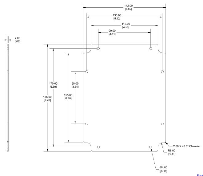
Enclosures can be Factory Modified (Milling, Drilling, Printing etc.) Contact Factory (modshop@hammfg.com) for quotes Solid models of this enclosure available in .stp or .x\_t (Part number and text placement/orientation on our products are subject to change, we do not recommend using them as a locating reference for modification purposes)
