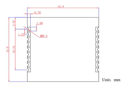
**Pic2. Module Dimension Diagram**
