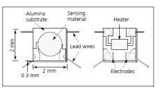
Fig 1a. Sensing element
