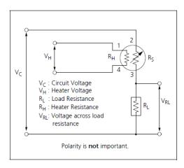
Fig 2. Standard circuit
