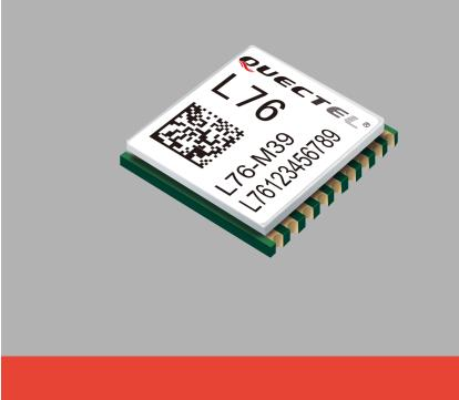
L76, the smallest GNSS module, is a single receiver module integrated GLONASS with GPS system. It provides simultaneous GPS and Compass GLONASS open service L1 reception capability. With 33 tracking channels, 99 acquisition channels, and 210 PRN channels, L76 can acquire and track any mix of GPS and GLONASS signals.
