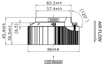
Assembly direction of customer's LED Module
