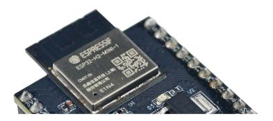
ESP32-H2-DevKitM-1 (with ESP32-H2-MINI-1 on board)
