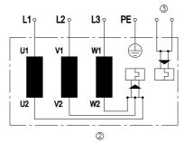
Change of rotation direction by reversing two phases
