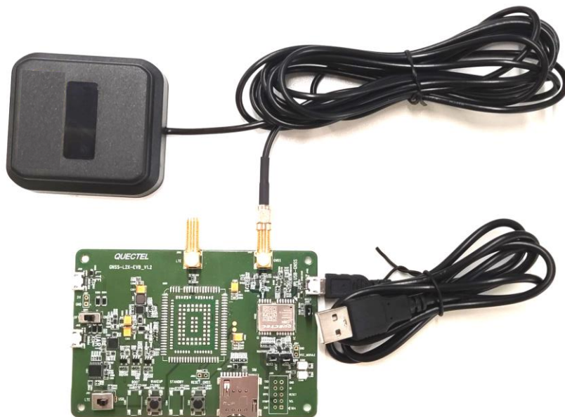
Figure 2: EVB and Accessories Assembly
