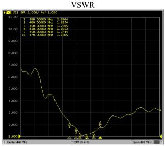
Tested with 250cm cable RG174 with SMA male
