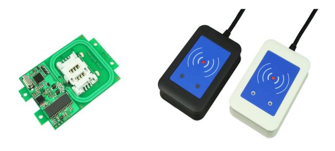
The TWN3 Multi ISO transponder Reader/Writer is designed for easy integration into various applications.
