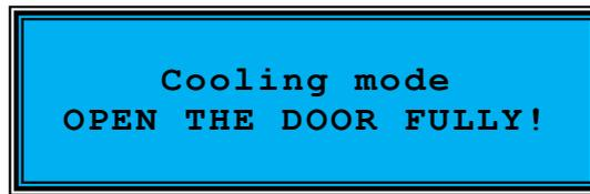
**ATTENTION!** This is very important for cooling down the oven. On the display, the oven informs and instructs the user about the necessity to open the door. After the oven has cooled down to the required temperature, which takes approximately 5 minutes, it is possible to unload the post-reflow PCB from the rack. Subsequently, the oven instructs the user to insert new PCBs, and the entire process is repeated as needed.
