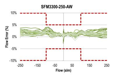
Figure 1. Exemplary flow-error of 30 units SFM3300-250-AW after autoclaving
