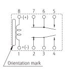
PC board mounting pad layout (TOP VIEW)
