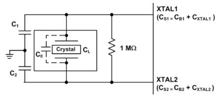
Figure 9.1 Typical Crystal Circuit
