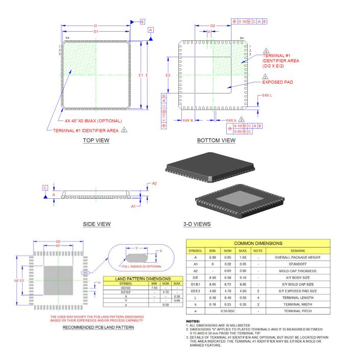
Figure 12.1 USB2660/USB2660i 64-Pin QFN
