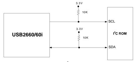
Figure 6.5 I<sup>2</sup>C Connection
