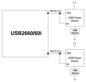
Figure 6.1 Port Power Control with USB Power Switch
