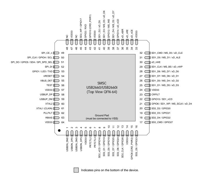
Figure 3.1 USB2660/USB2660i 64-Pin QFN
