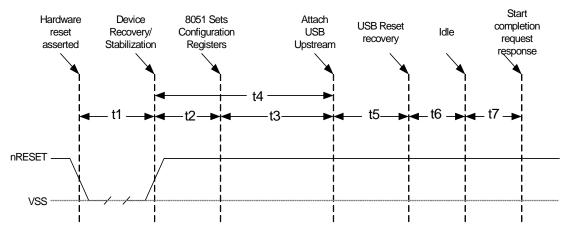
Figure 8.1 nRESET Timing for EEPROM Mode
