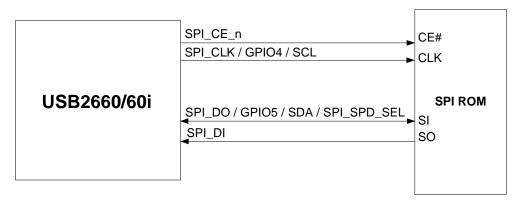
Figure 6.4 SPI ROM Connection
